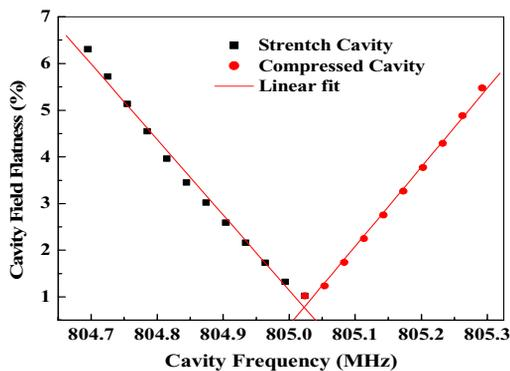
Figure 8: The simulation results of FF change with tuner-tuned frequency. The initial FF at free status is 1.32%.
