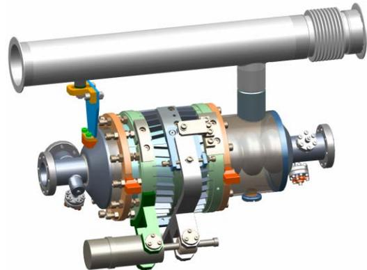
Figure 1: 3<sup>rd</sup> cavity, equipped with helium vessel and frequency tuner (design).
