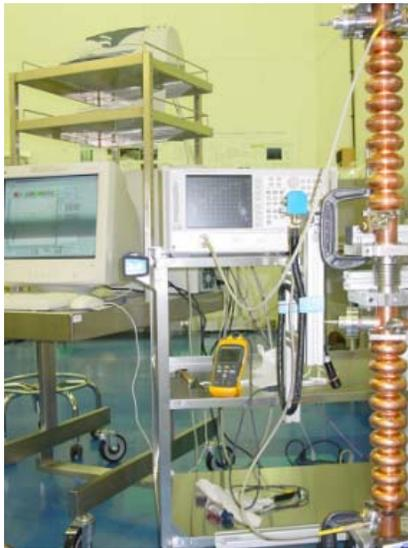
Figure 7: HOM studies of assembly of the two copper cavities on the bead-pull set-up in clean room.
