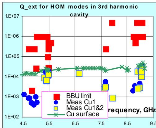
Figure 8: Q vs. frequency for HOM in TM<sub>010</sub> cavity. Red- BBU limit, blue&yellow – measurements, green-Copper.
