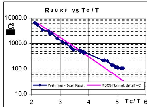
Figure 5: Surface resistance vs.  $T_c/T$  for CKM cavity.
