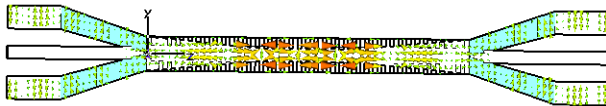
Figure 4: A snapshot of the traveling wave electric field fed to a structure with 30 inner cells is shown. The power is removed at the outlet by an identical coupler.
