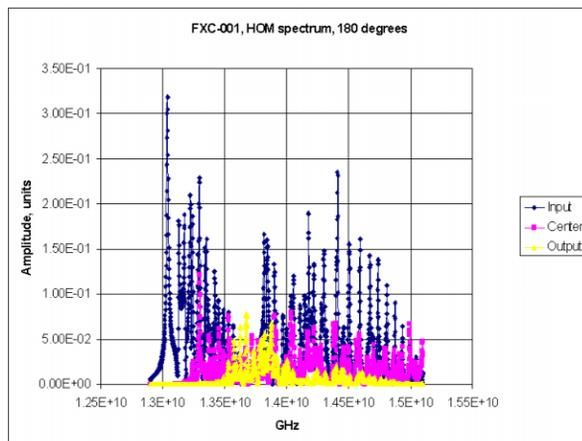
Figure 3: HOM spectra for different positions of probes.
