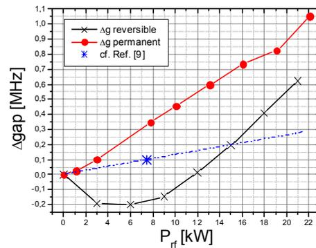
Figure 3: Permanent and reversible change of gap  $g$ .
