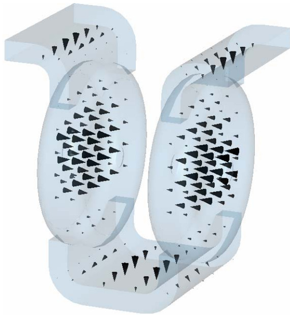
Figure 3: Electric field distribution for operation mode of the biperiodic structure.
