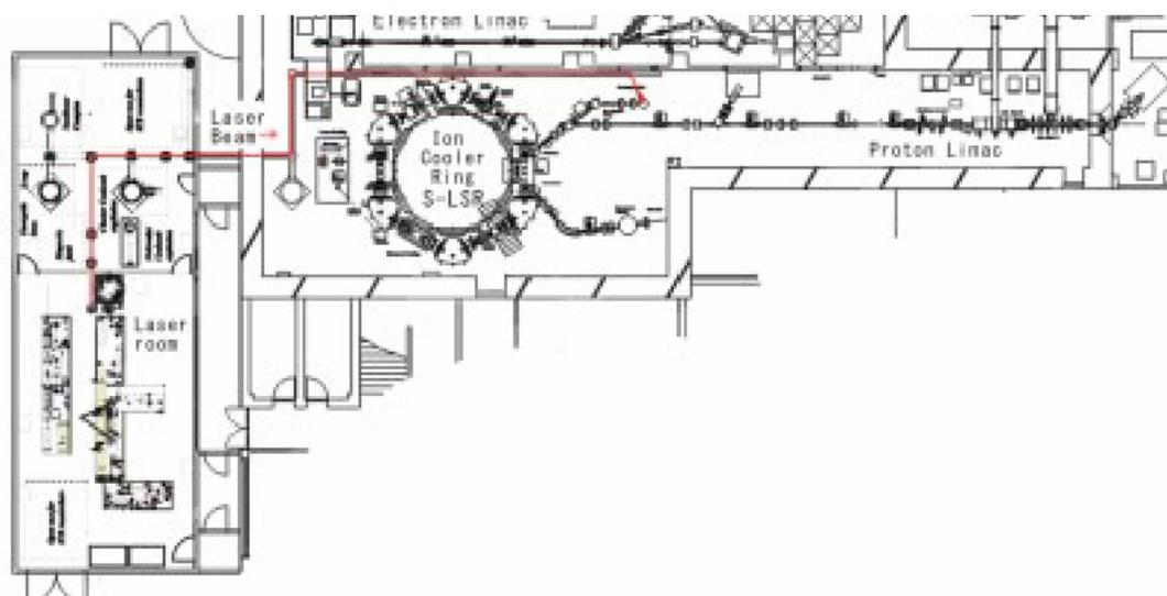
Figure 8: Layout of the combined facility of the accelerator and high power short pulse laser.
