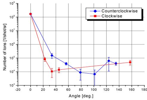
Figure 3: Angular distribution of laser produced protons.
