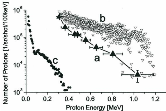
Figure 5: Energy distribution of laser produced proton in the direction of laser propagation. (a) experimental results, (b) simulation by under-dense plasma model, (c) simulation by over-dense plasma model [5].
