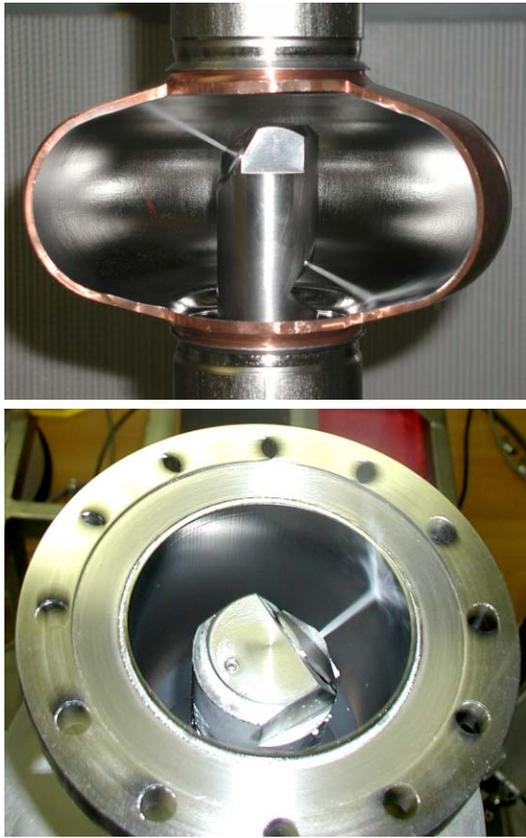
Figure 3: Nozzle test in a cut NbCu cavity (top) and in the beam tube of a Nb monocell (bottom).
