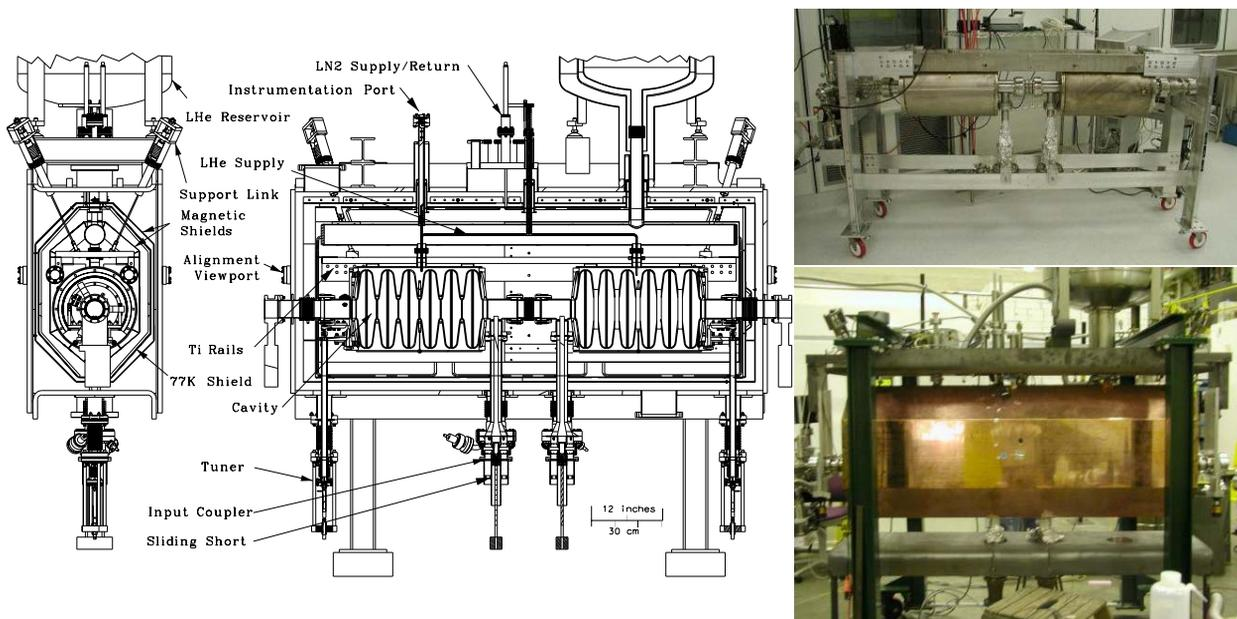
Figure 1 Left: end view and section view of the  $\beta = 0.47$  prototype cryomodule. Top right: cavities inside the helium vessels after attachment of the Ti rails and input couplers. Bottom right: Cold mass after installation of the thermal shield.
