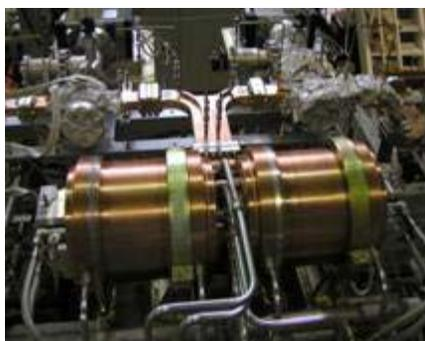
Figure 7: Whole view of the pulse compressor “SKIP” at test stand.
