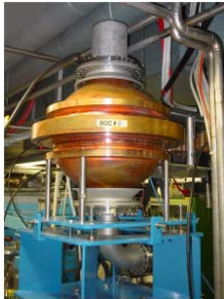
Figure 3: BOC pulse compressor.
