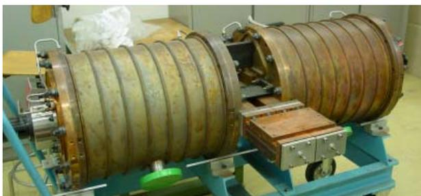
Figure 2: LIPS pulse compressor.
