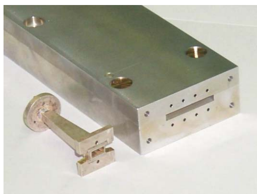
Figure 2: Mode launcher based on rectangular cross-section waveguide (photograph of the prototype).
