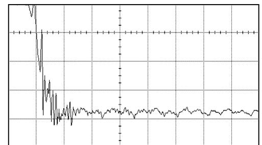
Figure 8: Transient voltage in the PFN connector (measured)
