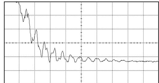
Figure 6: Transient voltage in the PSC In connector (measured)
