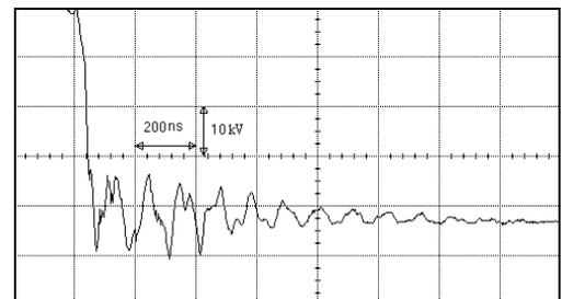
Figure 7: Transient voltage in the PSC Out connector (measured)
