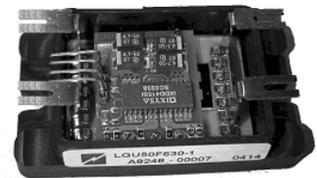
Figure 11: IGBT with gate drive 6.5kV.
