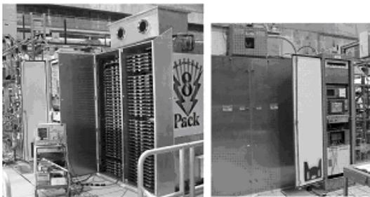
Figure 1: "8-pack" Solid State modulator installation.
