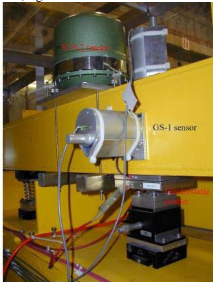
Figure 3: Close-up of sensors and electrostatic actuators.
