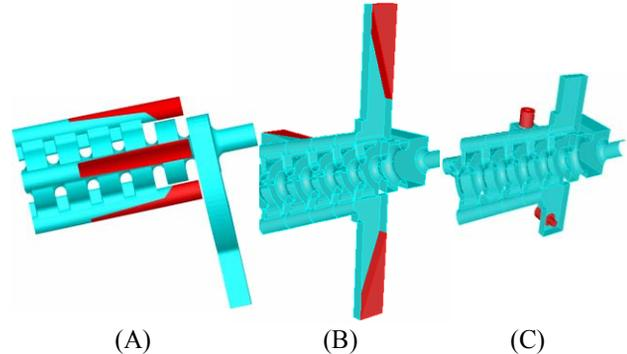
Figure 10: Three types of HOM coupler design.
