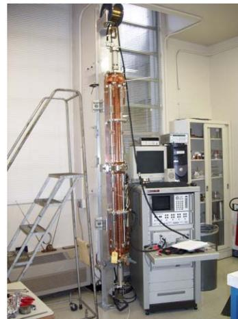
Figure 11: Wire measurement set-up with the RDDS1 structure.
