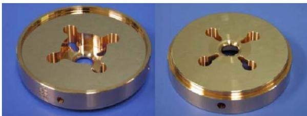
Figure 4: View from both sides of an accelerator cup.
