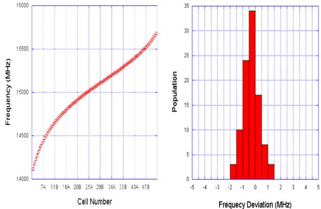
Figure 5: Measured dipole mode frequencies (left) and their tolerances.
