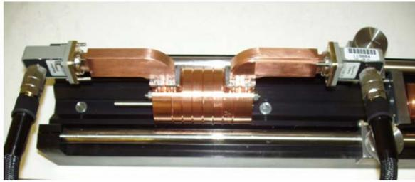
Figure 7: Microwave measurement for a HOM coupler test assembly.
