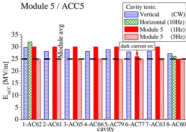
Figure 4e: Single cavities tests: ACC5.
