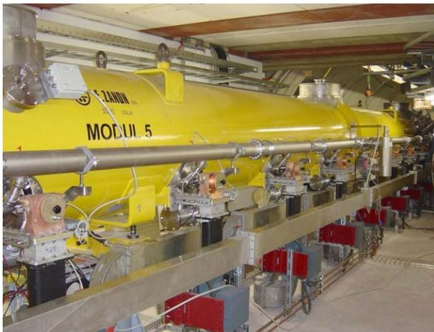
Figure 2: Accelerating module in the VUV-FEL tunnel.
