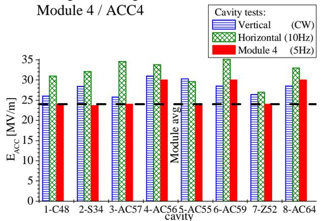
Figure 4d: Single cavities tests: ACC4.
