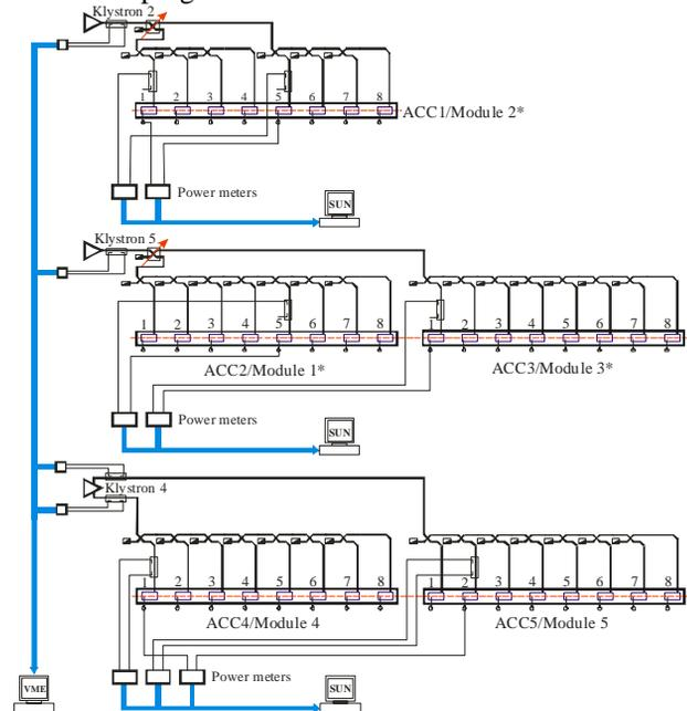
Figure 3: RF power distribution / measurement diagram.
