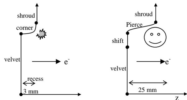
Figure 1: Cathode geometries: a: Standard; b: Pierce.
