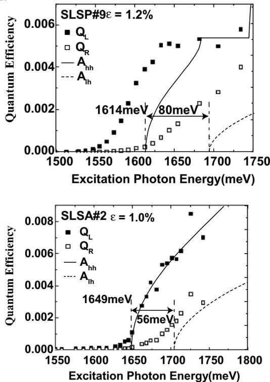
Figure 4: The  $Q_L$  and  $Q_R$  spectra (experimental) and the JDOS-based  $A_{hh}$  and  $A_{lh}$  spectra for SLSP#9 and SLSA#2.
