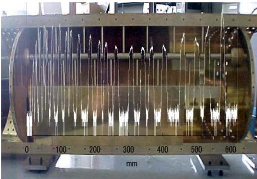
Figure 4: The electric field distribution by model test.
