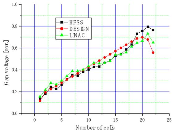
Figure 6: Comparison of the gap voltage distribution.
