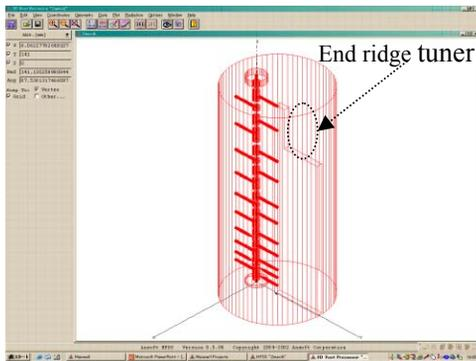
Figure 3: End Ridge tuner length=120mm by H.F.S.S.
