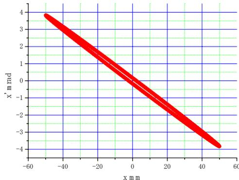
Figure 7: Emittance from the ion source.
