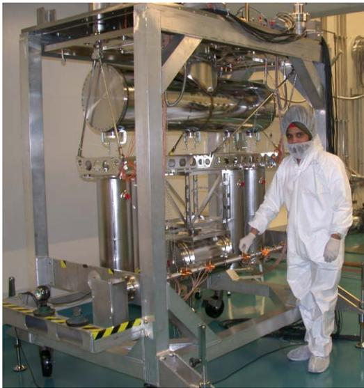
Figure 2: Top plate assembly in assembly stand.
