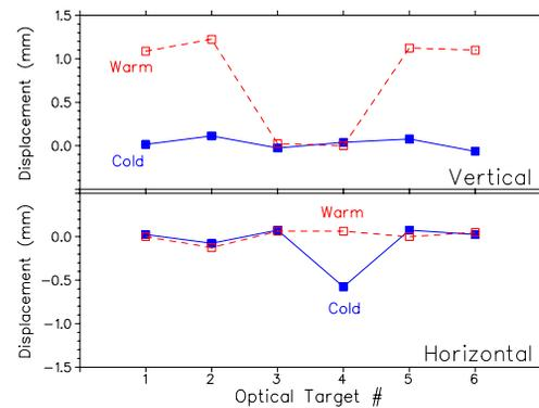
Figure 5: Measured positions of the six optical targets relative to their specified positions for warm and cold conditions.
