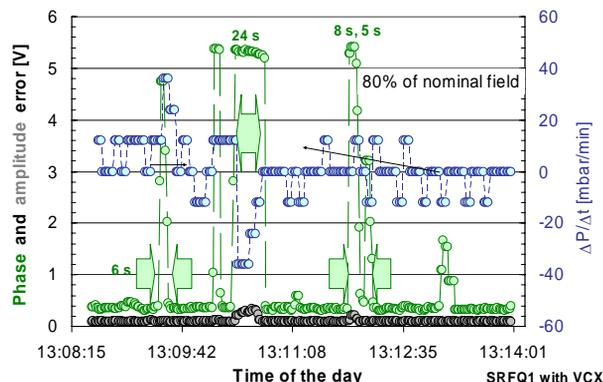
Figure 3: Samples of locking and out-of-lock periods of SRFQ1, with the VCX fast tuner and 80% of the nominal field. Every second, the maximum of  $|\Delta\phi|$  and  $|\Delta A|$  detected in the last 400 ms is shown on the graph.
