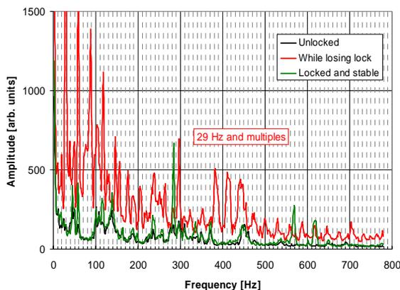
Figure 4: Spectra were taken on the suspension bar of SRFQ2 in three conditions: out-of-lock cavity (black line); stable locked cavity (green line); transition period during which the cavity is losing lock (red line).
