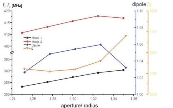
Figure 9: Mode frequencies, Dipoles and Q as function of the aperture radius.
