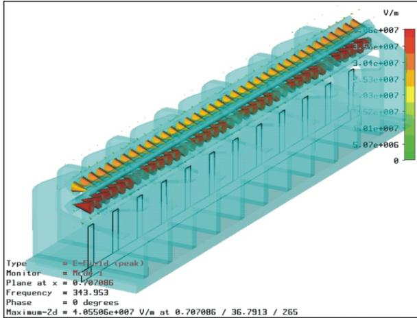
Figure 7: Electric field distribution in the  $\pi_0$ -Mode.
