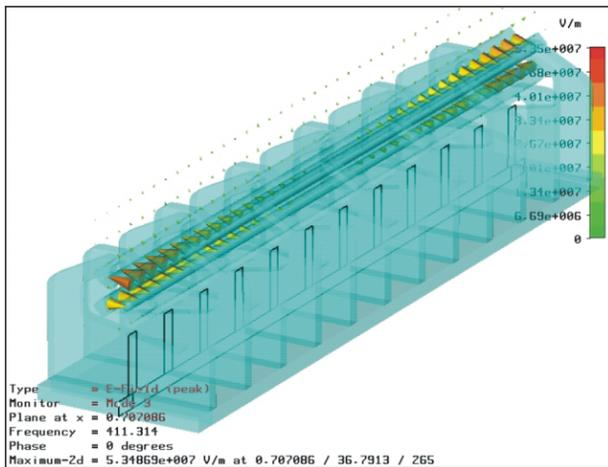
Figure 8: Electric field distribution in the  $\pi_1$ -Mode.
