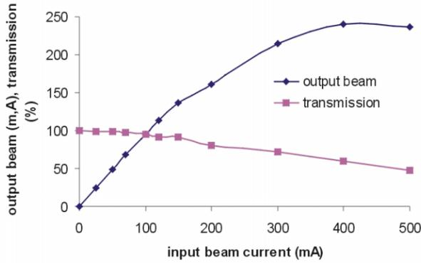
Figure 3: RFQ output proton current as a function of the input proton beam current. Transmission as function of the input beam current.
