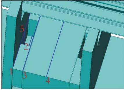
Figure 8: RFQ tuning block between stems with a short central slot (30mm).
