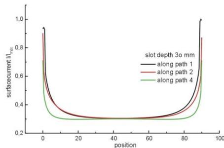
Figure 6: current distribution across the RFQ-cell at different points.
