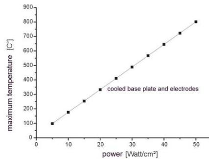
Figure 12: Maximum temperature in a RFQ cell with constant power/area. Base plate and electrodes are cooled.
