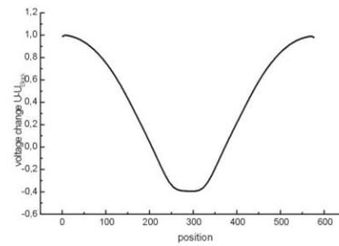
Figure 4: Electrode field changes induced by the central tuning block.
