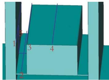
Figure 5: RFQ tuning block between stems with slots.
