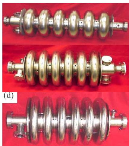
Figure 2: Examples of  $\beta=0.81$ , 0.61, and 0.47 elliptical cavities [27, 35]
