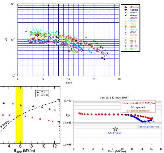
Figure 7: Experimental results for TM-class elliptical cavities (upper) and TEM-class spoke cavities (lower).
