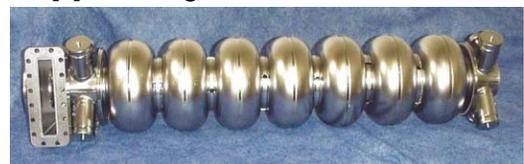
Figure 2: LL seven cell cavity.
