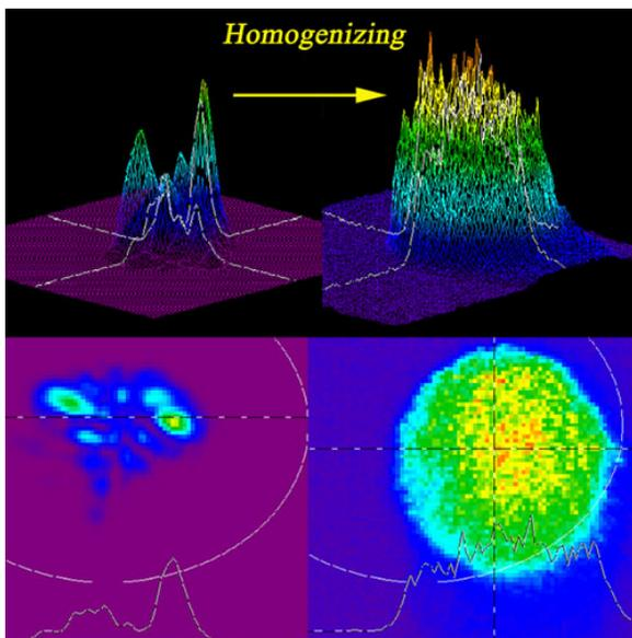
Figure 3: Homogenization results with microlens array.
