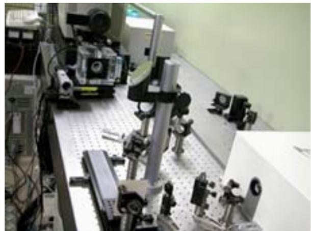
Figure 2: Adaptive-optics complex for shaping both spatial and temporal laser profiles.
