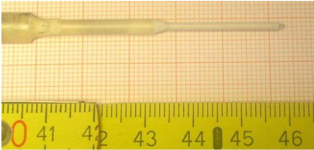
Figure 3: Ceramic shielded probe with tip
