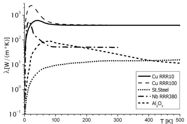
Figure 5b: Thermal Conductivities with Temperature.
