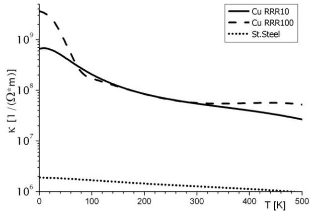
Figure 5a: Electrical Conductivities with Temperature.
