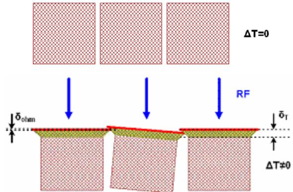
Figure 3: Interaction of grains under pulse RF heating.
