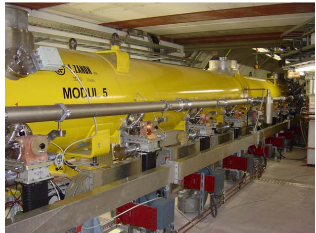
Figure 4: Module ACC 5 equipped with the TTF 3 couplers. Above the couplers the common pumping line for all 8 couplers is seen. Below the couplers the wave guide distribution system with the remote controlled three stub wave guide tuners, directional couplers and circulators is assembled.
