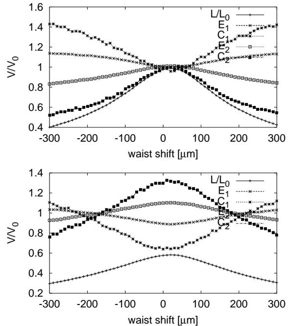
Figure 1: Examples of the waist optimisation. In the upper plot, the waist of beam 2 is in optimum position and beam 1 is scanned. The variables  $E_i$  and  $C_i$  are the beamstrahlung and coherent pair power of beam 1 and beam 2, respectively. The coherent pair power gives a more pronounced signal. In the lower plot, beam 2 has a waist shift of  $200\mu\text{m}$ .
