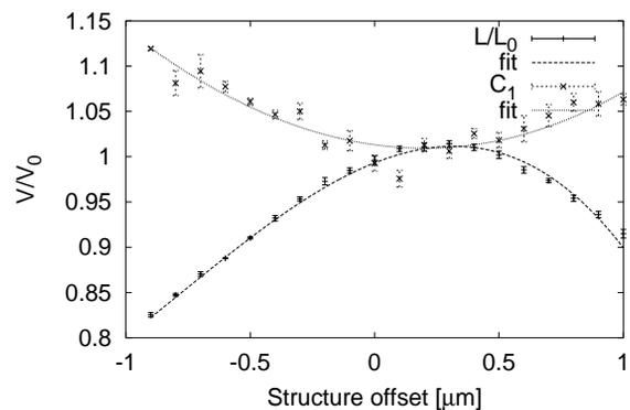
Figure 2: Example of the optimisation of a main linac bump for beam 1. The luminosity (normalised to the mean of the 50 different machines) and the coherent pair power of beam one are shown (also normalised to the mean of 50 machines). The error bars were derived running the same case five times using different seeds for the random number generators.
