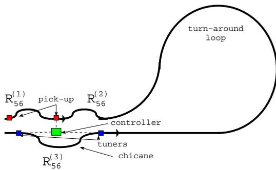
Figure 3: An example layout of a phase feedback.
