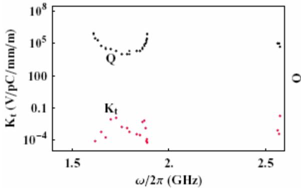
Figure 2: Calculated transverse kick factors and measured Q values for TESLA accelerating cavities.
