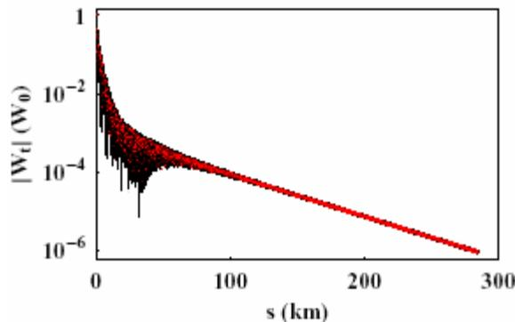
Figure 3: Envelope of the TESLA transverse wakefield. The abscissa runs over the distance of the complete bunch train. The ordinate has been normalized with respect to  $W_0$ , (0.11 V/pC/mm/m). The red dots indicate the location of the individual bunches.
