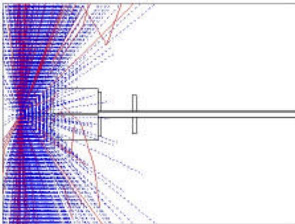
Figure 3: (a) Background from electrons hitting internal part of the undulator, (b) background from electrons hitting the collimator: blue – photons, red - electrons and positrons.
