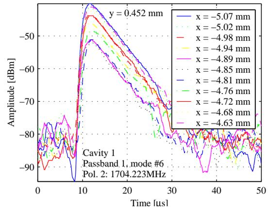
Figure 4: Time domain signals for the first polarization of the 6<sup>th</sup> mode of the 1<sup>st</sup> dipole band of the first cavity.
