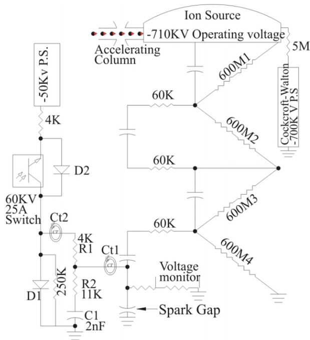
Figure 2: Block diagram of bouncer and coupling network.
