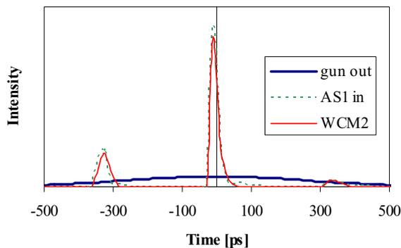
Figure 2: Bunching of the beam in short-pulse mode.
