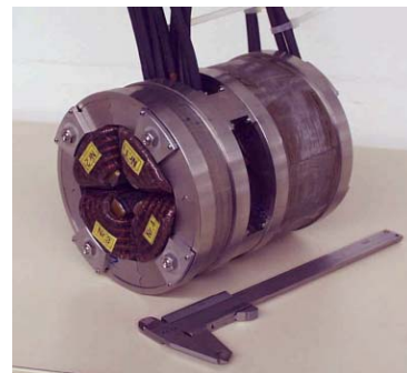
Figure 3: Prototype quadrupole doublet built at GSI [14]. The yoke lengths are 42 mm and 81 mm. The distance between the yokes of the two magnets is 27 mm only.
