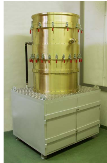
Figure 5: View on the 1.4 MW final stage cavity amplifier after delivery to GSI. The outer diameter of the system is 980 mm, the total height 2595 mm. (Photo by G. Otto, GSI; published with great acknowledgements to Dr. Klaus Berdermann, BERTRONIX Electronic GmbH, Munich, Germany.)
