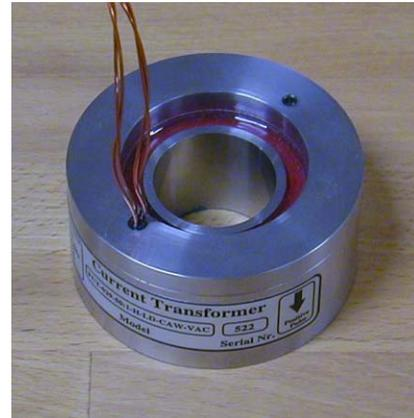
Figure 1: SNS transformer for the DTL section.
