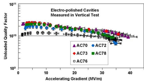
Figure 6: Recent test results for electro-polished TESLA cavities.
