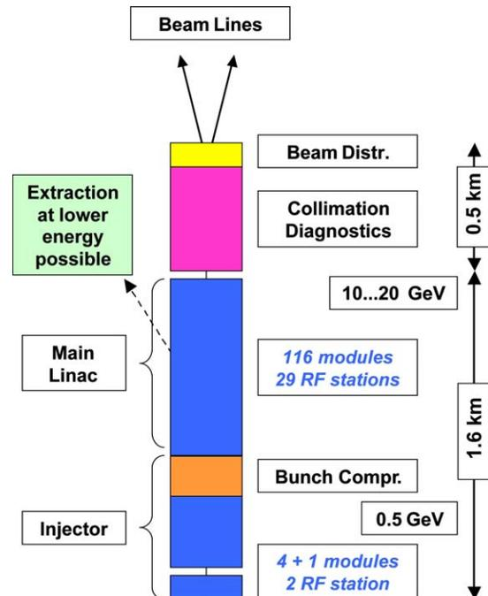
Figure 3: Basic Layout of the XFEL Accelerator.
