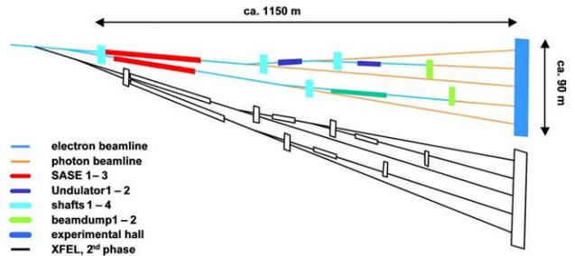
Figure 2: The 1<sup>st</sup> stage user beamline layout (coloured) and the possible extension.
