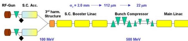
Figure 7: XFEL Injector Layout.
