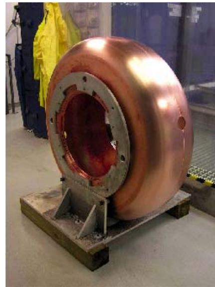
Figure 5: 201 MHz cavity being fabricated at Jlab. The beam aperture is 420 mm in diameter, and the cavity body is about 1.2 m in diameter. The small hole visible on the side is a pilot hole for extruding one of the four required equatorial ports.
