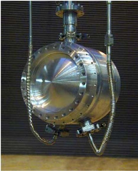
Figure 6: Prototype LH<sub>2</sub> absorber developed at KEK and successfully tested at the Fermilab MTA.
