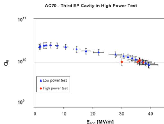
Figure 1: 35MV/m result of AC70 EP cavity.
