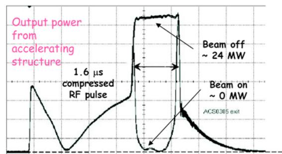
Figure 6: Beam loading of CTF3 injector structure.
