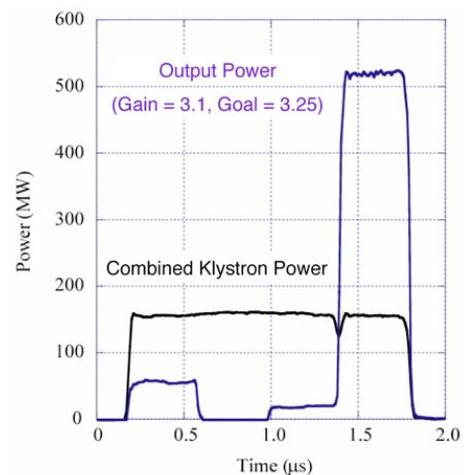
Figure 3: 510MW, 400ns power from 8-pack system.
