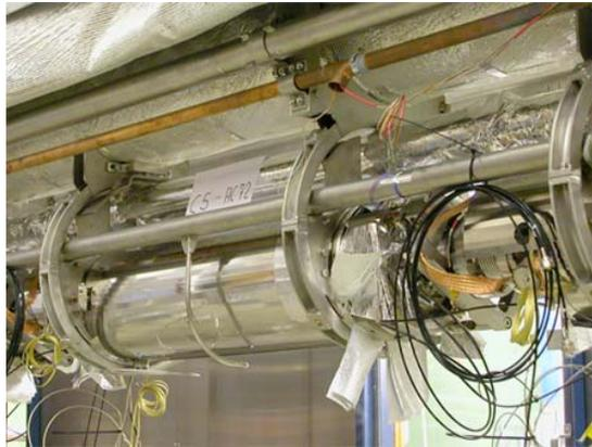
Figure 2: 35MV/m AC72 cavity installation.
