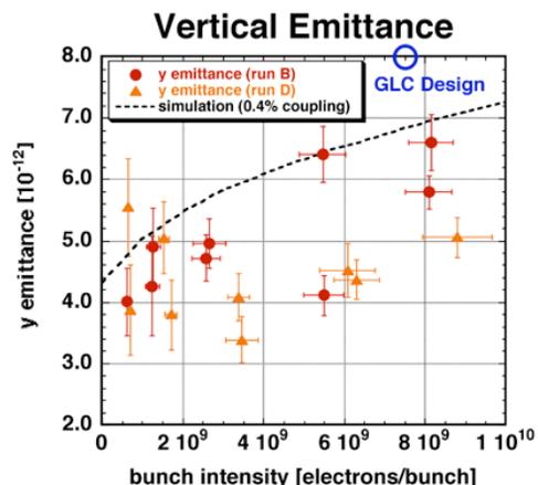
Figure 5: ATF vertical emittance in single bunch.
