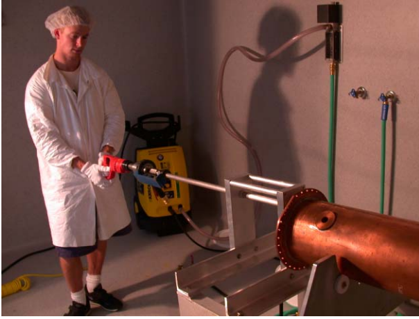
Figure 3: The manual high pressure water rinse system shown with the copper 'dummy' cavity.
