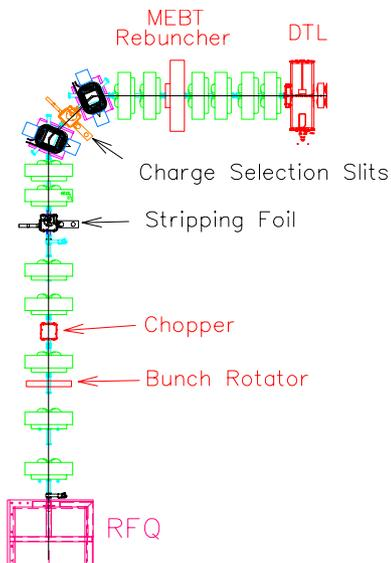
Figure 1: ISAC Medium Energy Beam Transport (MEBT).
