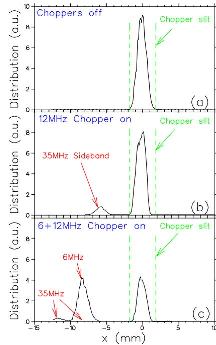
Figure 4: Measured beam profiles at the chopper slit for (a) chopper off (b) chopper Mode A and (c) chopper Mode B.
