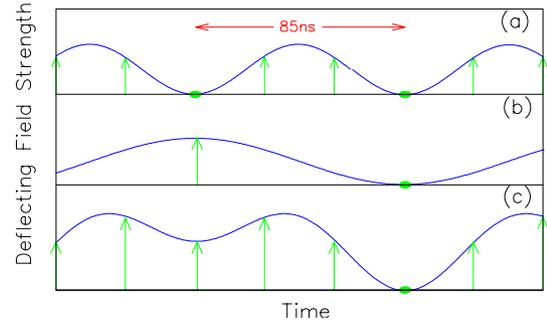
Figure 3: A schematic of the two-mode tandem chopper waveforms. For Mode A the first set of plates is excited with an 11.7 MHz deflecting voltage as is shown in (a). For Mode B the second set of plates is also excited at 5.8 MHz as shown in (b). The total resultant deflection for Mode B is shown in (c).
