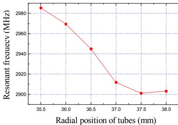
Figure 2: Variation of the resonant frequency as a function of location of the support tubes.
