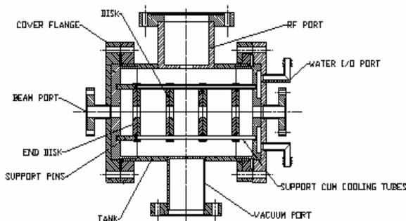
Figure 1: Schematic of the prototype, 4-cell, PWT linac structure.
