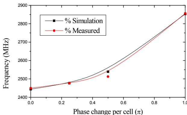
Figure 6: Dispersion curves for the PWT structure.
