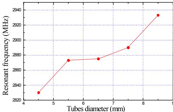
Figure 3: Variation of the resonant frequency with tube diameter, for a fixed PCD of the tubes.
