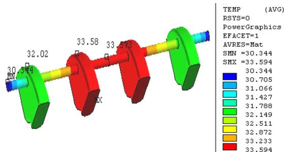
Figure 4: Steady-state temperature profile of the disk-array with copper rods.
