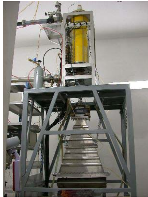
Figure 14: 4.5 MeV electron linac for protecting mail against anthrax.
