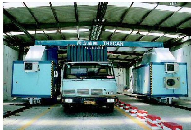
Figure 9: Relocatable type container inspection system
