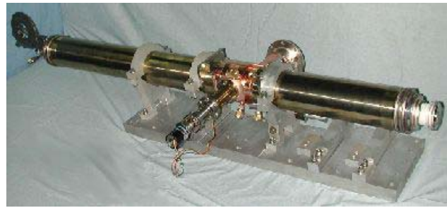
Figure 4: 20MeV SW medical acceleration tube with an energy switch.
