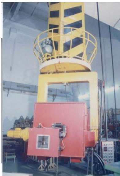
Figure 11: 9MeV electron linac for radiography
