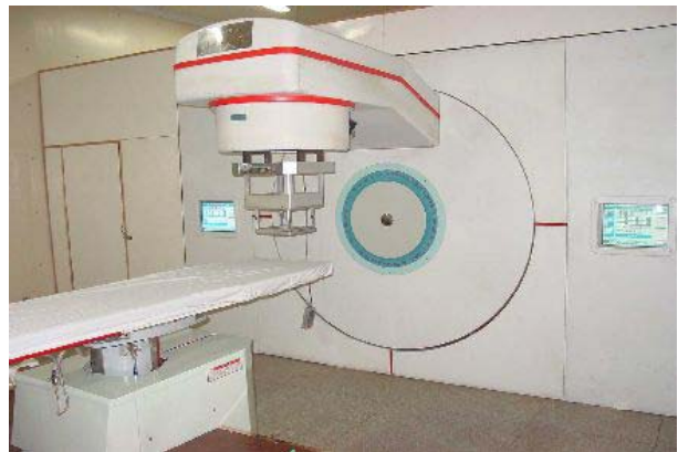
Figure 5: 16MeV medical travelling-wave electron linac.
