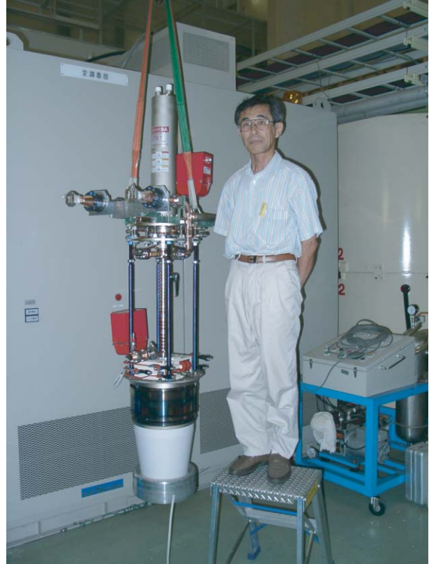
Figure 4: X-band PPM Klystron developed at KEK
