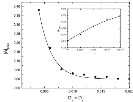
Figure 3: Variation of the radiation amplitude peaks according to the radiation domain. The peaks exponentially decrease as the domains increase. (inset: Amplitude peaks according to the radiation wavelength. The peaks show a monotonic increment as the wavelength increases.) (Solid curve is for eye guide).
