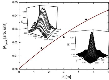
Figure 2: Variation of the radiation amplitude peaks according to the axial distance. The peaks monotonically increase along the axial distance (Solid curve is for eye guide). [Inset: Typical shape of radiation amplitude computed by using Gauss-Hermite (up) and Gauss (down) beam profiles.]
