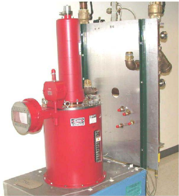
Figure 6: VKL-7966A Klystron in Electromagnet (Photo courtesy of TJNAF)
